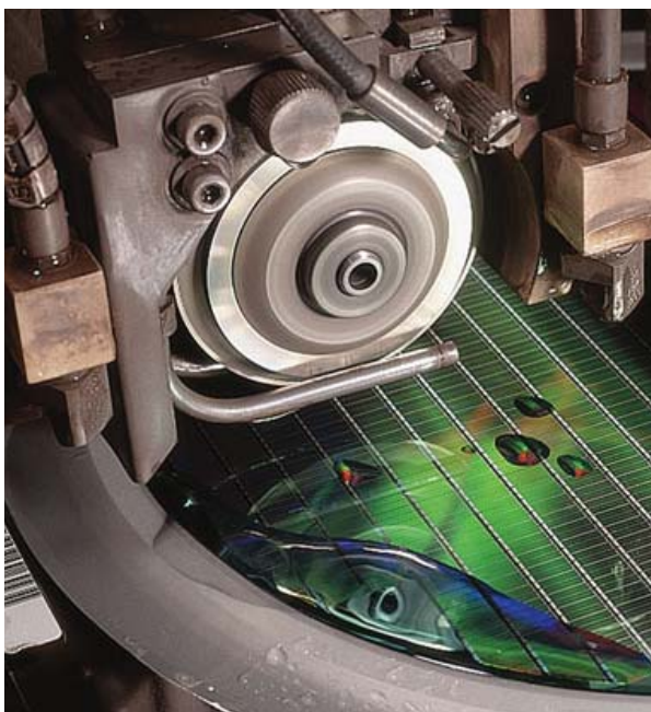
Die cutting process: One of the several hundred crucial steps in turning a wafer into a finished chip.
