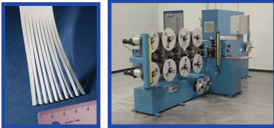
Fig. 2. (left) 4 cm wide strip of silver-coated HTS strip roll-slitted to ten 4 mm wide wires. The outer two are discarded because of edge non-uniformities in the original MOD coating process. (right) Roll slitting apparatus
