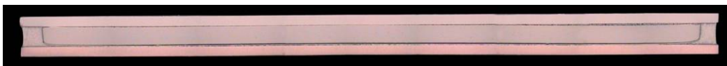
Fig. 3. Cross section of 344 superconductors: a 2G HTS wire with a substrate, thin buffer/HTS/Ag layers and two copper laminates.
