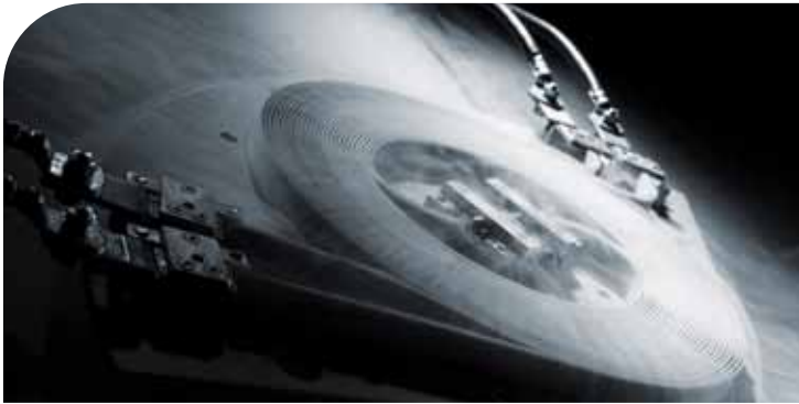
FCL module containing coils of superconductor wire
