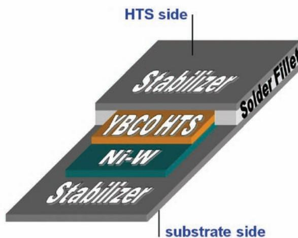
Figure 1. Structure of Amperium wire
