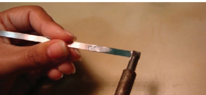
Figure 5. Tinning the wire end. Start with the iron away from the wire end (a) and work the solder layer towards the end (b) to produce a smooth, even coating.
