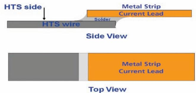
Figure 3. HTS wire – metal strip current lead connection
