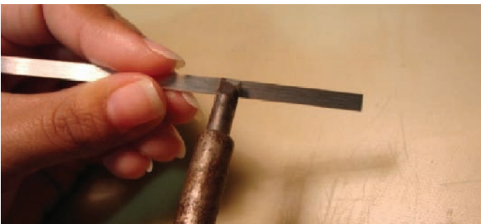
Figure 7. Tinned and cleaned HTS wire and metal current lead
