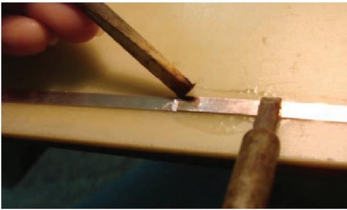
Figure 10. Soldering the wire and metal lead together
