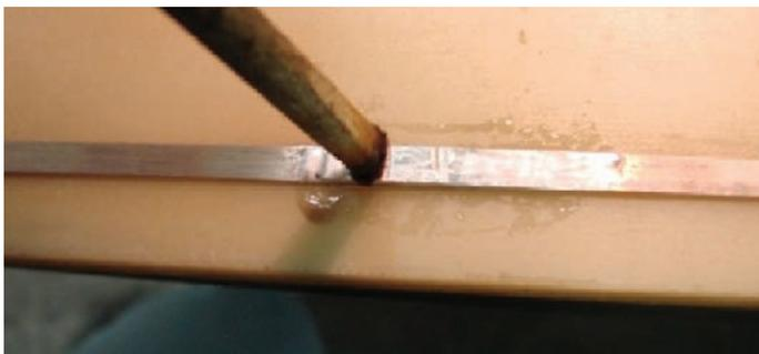
Figure 11. Maintaining pressure on joint as it cools.
