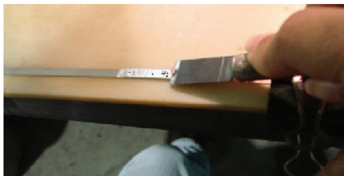
Figure 12. Gently removing excess solder with an Xacto knife
