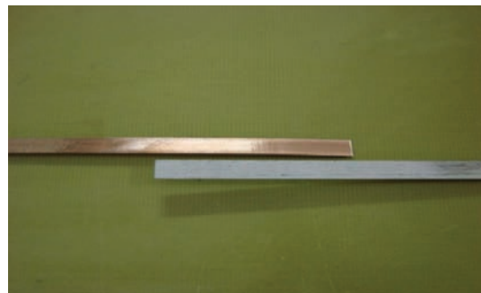
Figure 7. Tinned and cleaned HTS wire and metal current lead
