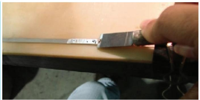
Figure 12. Gently removing excess solder with an Xacto knife
