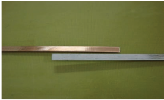
Figure 4. Cut HTS wire and copper lead ready for soldering
