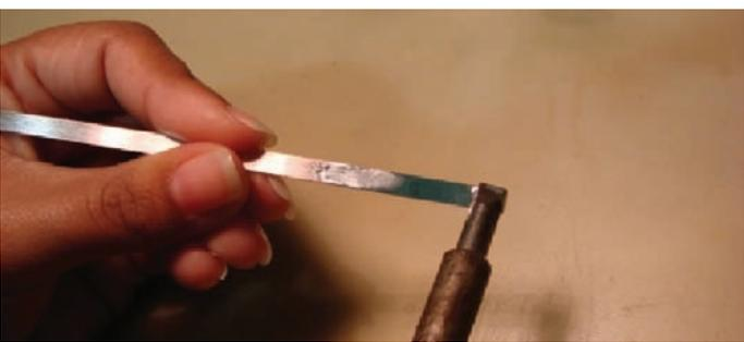
Figure 5. Tinning the wire end. Start with the iron away from the wire end (a) and work the solder layer towards the end (b) to produce a smooth, even coating.
