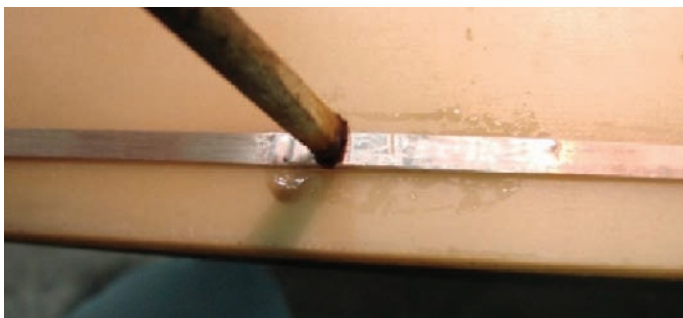
Figure 11. Maintaining pressure on joint as it cools.
