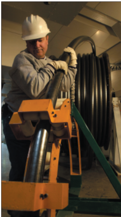
Fig. 3 — High temperature superconductor wire allows power cables to be manufactured that can support up to ten times the capacity of conventional cables based on copper wire. They support load growth, enable cost-effective controllability of power over a meshed grid, and can be implemented with low environmental impact. Liquid nitrogen, the dielectric and coolant of choice to maintain HTS wire at its operating temperature, is inexpensive, abundant, and environmentally safe — eliminating the oil currently used in many conventional power cables.
