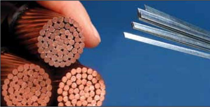
Superconductor wire conducts more than 100 times the electrical current of equivalent sized copper wire. The wires on the right carry as much power as all of the copper on the left. Courtesy of American Superconductor
