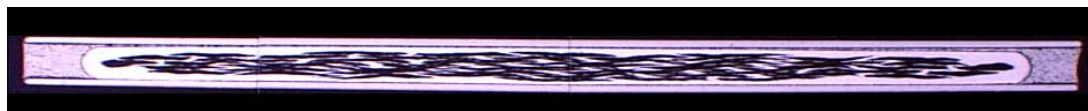
Figure 5. Cross-section photomicrograph of Hermetic Wire showing thin strips of stainless steel on the top and bottom of the tape and solder fillets on the left and right of the tape.
