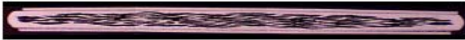
Figure 3. Cross-section photomicrograph of High Strength wire showing 37 \mu\text{m} thin strips of stainless steel on the top and bottom of the tape.
