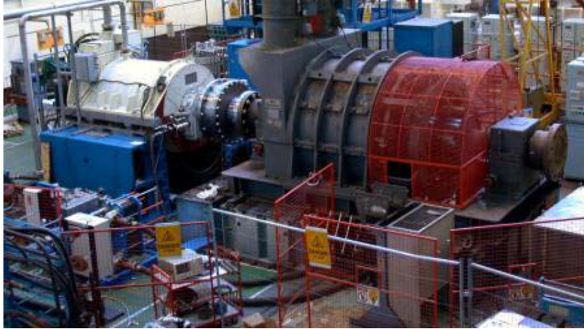
Figure 9: 5 MW HTS Motor (left) connected to a 2.5 MW conventional generator on a factory test stand.
