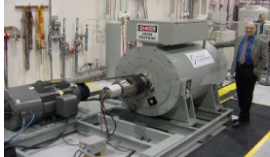
Figure 5: AMSC 5000 hp motor under test
