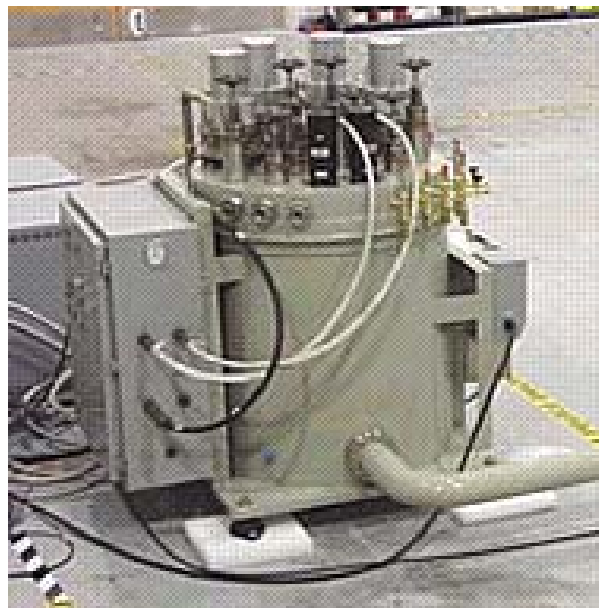
Figure 11: Cooling system built for 5 MW, 230-rpm motor
