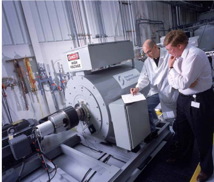
Figure 12: Single-layer stator armature employed in AMSC built 5000 HP, 1800-rpm, 4 pole motor
