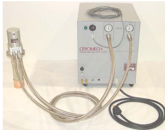
Figure 9: A Cryomech cryocooler cold head and its compressor
