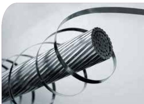
AMSC's Amperium wire wound around a copper bundle with equivalent current carrying capability. Amperium wire conducts more than 100 times the electrical current of equivalent sized copper wire.
