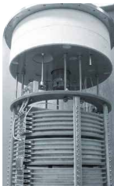
FCL Coil with AMSC's Amperium Stainless Steel Wire.
