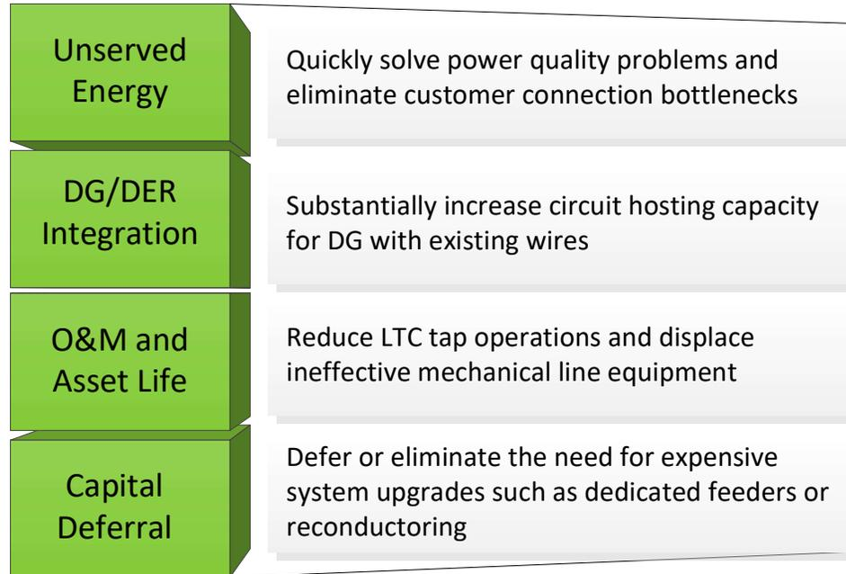
Figure 1. Value stack for D-VAR VVO applications.
